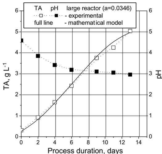
Fig. 4. Changes in pH values and titratable acidity in large reactor compared to the calculated acidity.
