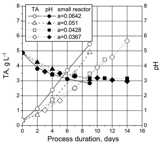
Fig. 3. Changes in pH values and titratable acidity in small reactors.
